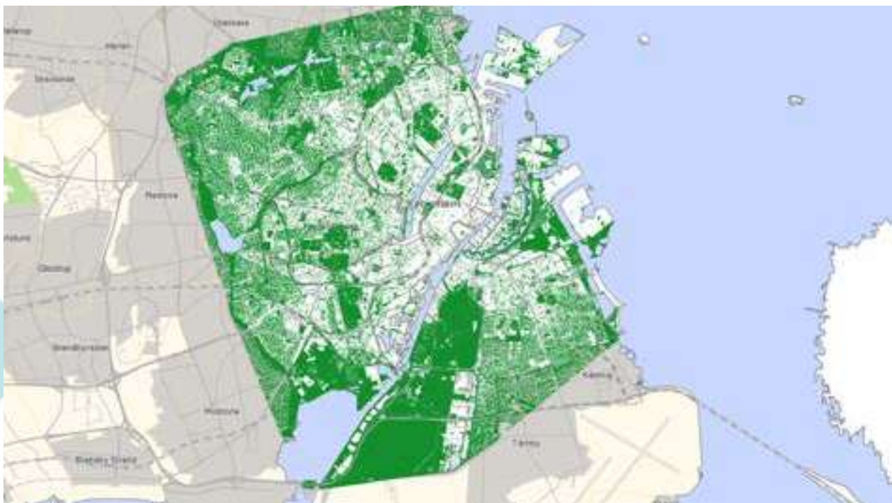
The result of a NDVI analysis. Areas with vegetation stand out and have been colorized with a green tint.
