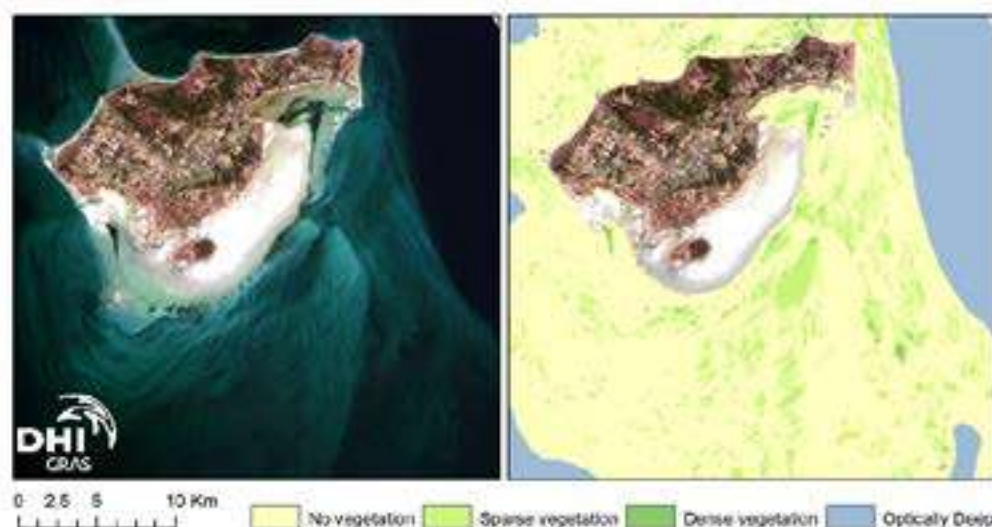
Satellite-derived mapping of submerged aquatic vegetation around the Danish island of Laesoe.
