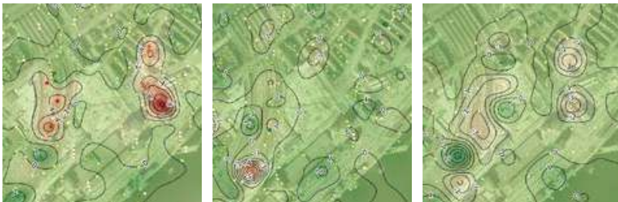
Figure 1. Vertical movement calculated from calibrated Sentinel-1 LOS data for ascending track LOS-146A (top) and LOS-66D (middle). The vertical movement is shown as a 2D product (bottom).
