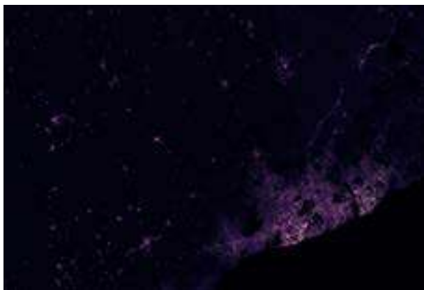
Processed map of surface structures in the capital region - 'Greater Accra Region'. The image is a combination of Sentinel-1 Coherence and Backscatter.
