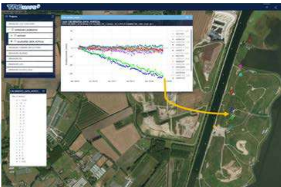
The inSAR measurement points on Stige Ø north of Odense supported the presumption that the area was subsiding and enabled the municipality to estimate the rate and total level locally.
