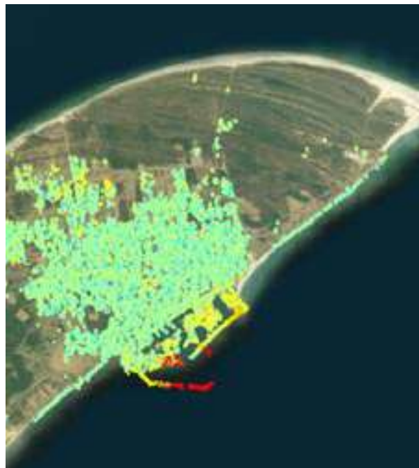
In Denmark, millions of point scatterers have allowed for estimating the deformations of e.g. houses, railways and harbours. Here, the town of Skagen is displayed in a simple colour code. Ref.: TRE Altamira (2019).
