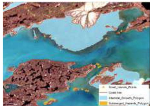
Mapping intertidal zones, coastline extent, small islands and submerged hazards using Sentinel-derived data composites.
